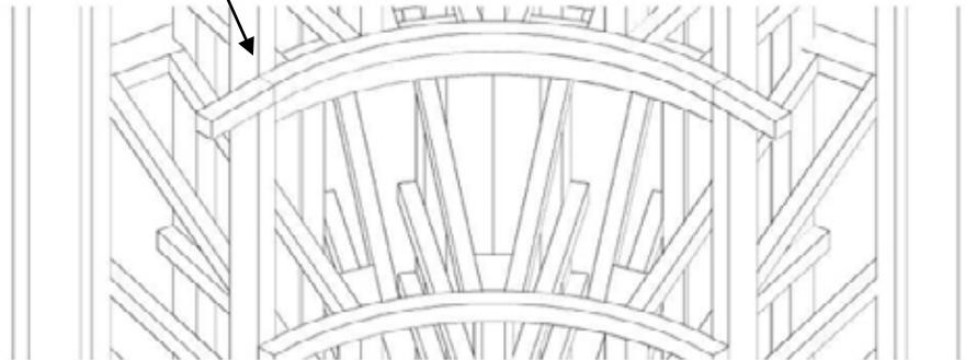
8. Repeat steps 6 and 7 to attach the remaining six (five for Classic height) curved front spacer bars, as shown in Figures 4 and 5.
