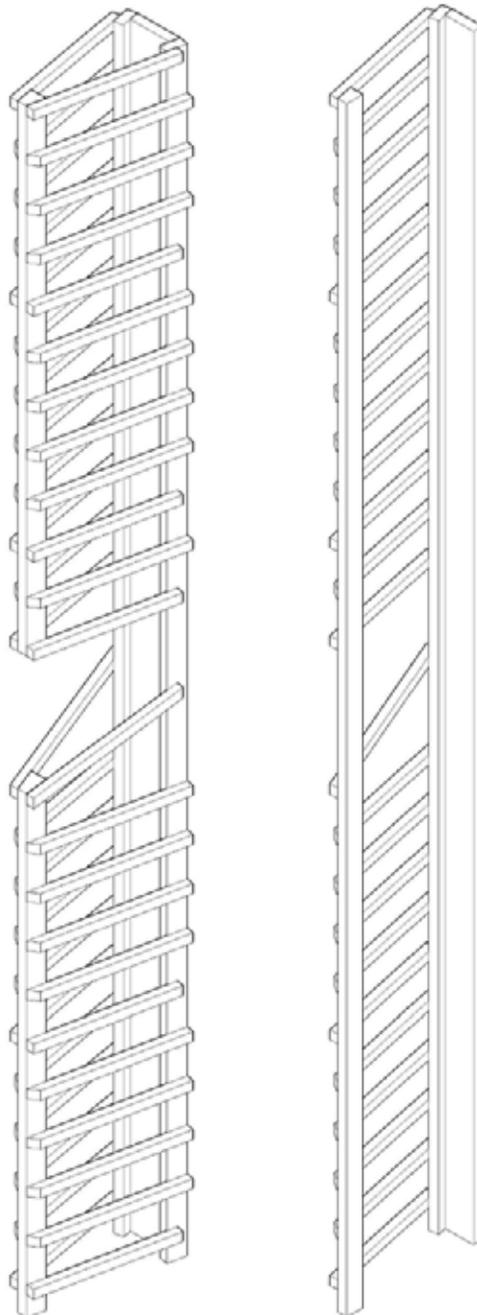
2. Take one of the pre-drilled back spacer bars and position it at the middle spacer bar location, just above the angled display slats (See **Figure 2**). Pre-drill into the uprights using the 9/64" drill bit and attach with two screws provided.
