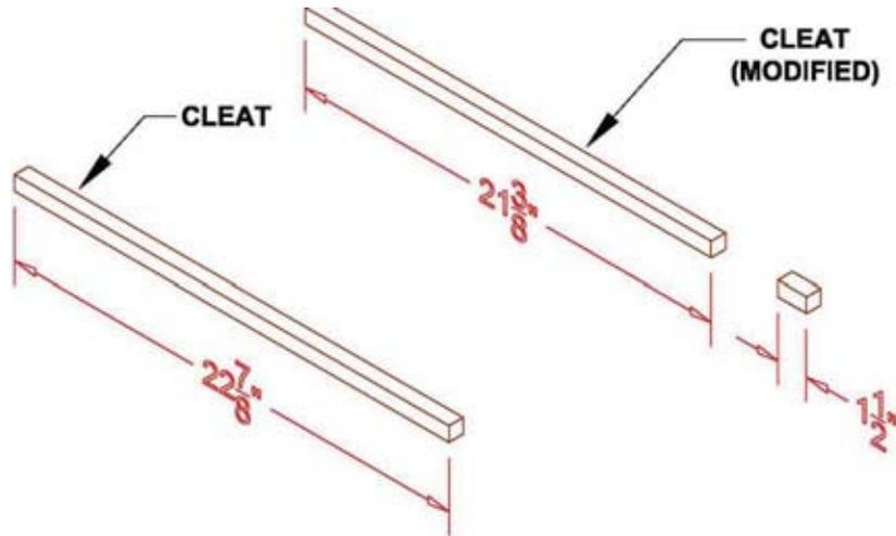
4. Insert the cleat into the top of your conversion box. Secure by nailing through the top of the conversion box and into the cleat using finish nails (not provided) (**Figure 4**). Make sure your nails are shorter than 1 1/2" long or they will go through your cleat and show in your conversion box.
