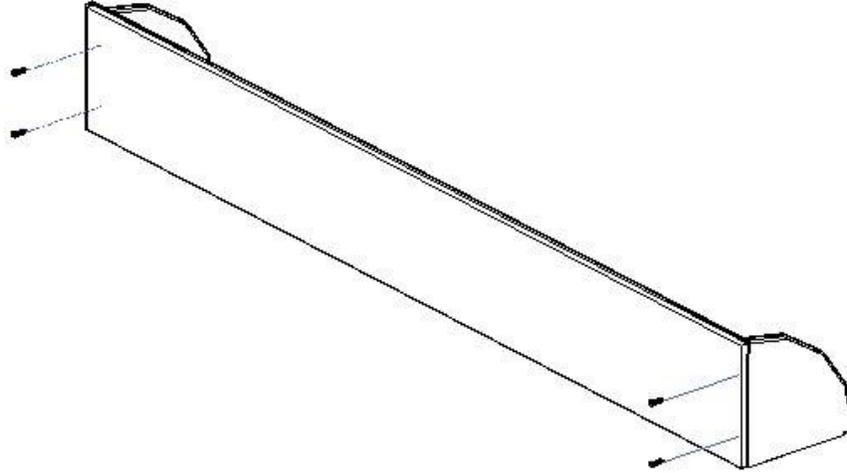
2. Turn the unit onto the side you just affixed and screw the back panel (wider width) to the top and bottom panel (See Figure 45).
