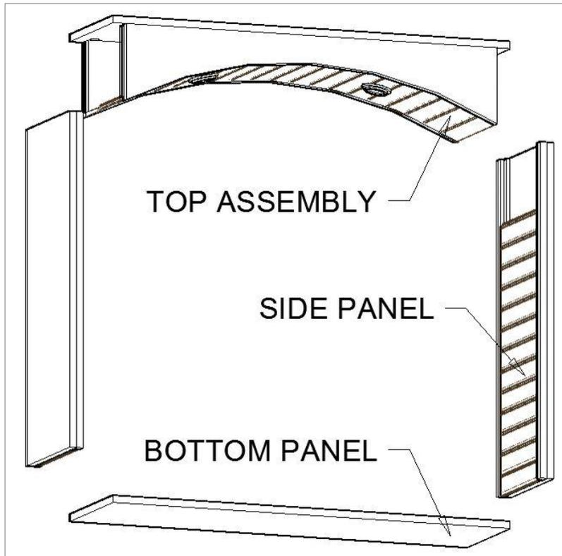
Arch Tops are constructed from 2 side panels, a top assembly and a back panel. **Note: There will be no bottom panel if you already have a predetermined table top the arch is connecting too.** If you have ordered an arch top with installed lighting please make note of the transformer location. Another hole may need to be drilled depending on the location of the outlet the transformer will plug into. Vigilant recommends the use of a licensed electrician when making all electrical connections.
