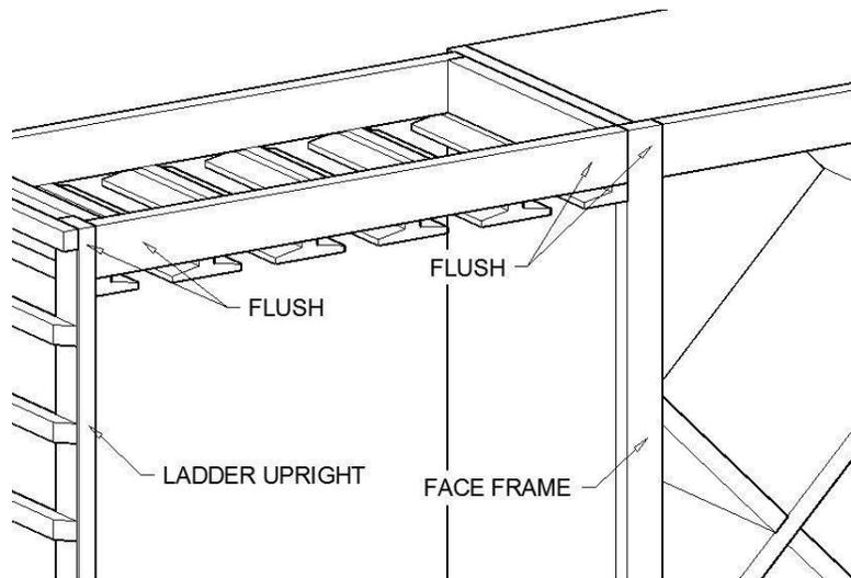
2. Pre-drill through the adjacent unit(s) into the sides of the unit. Affix with screws, and remove clamps.
