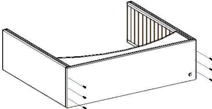
4. Screw through the side panels into the ends of the top assembly (See Figure 51).
