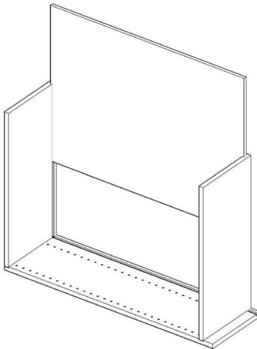
4. With the unit positioned on its side, repeat step 2 for the other side panel.
