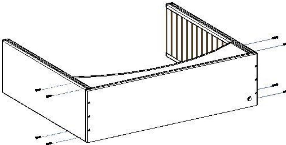
5. Repeat step 3 if a bottom panel was designed, if not the arch will sit directly on top of the finished table surface (separate component).
