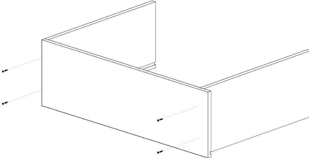
3. Turn the unit onto the side that you just assembled and insert the back panel (See Figure 38).
