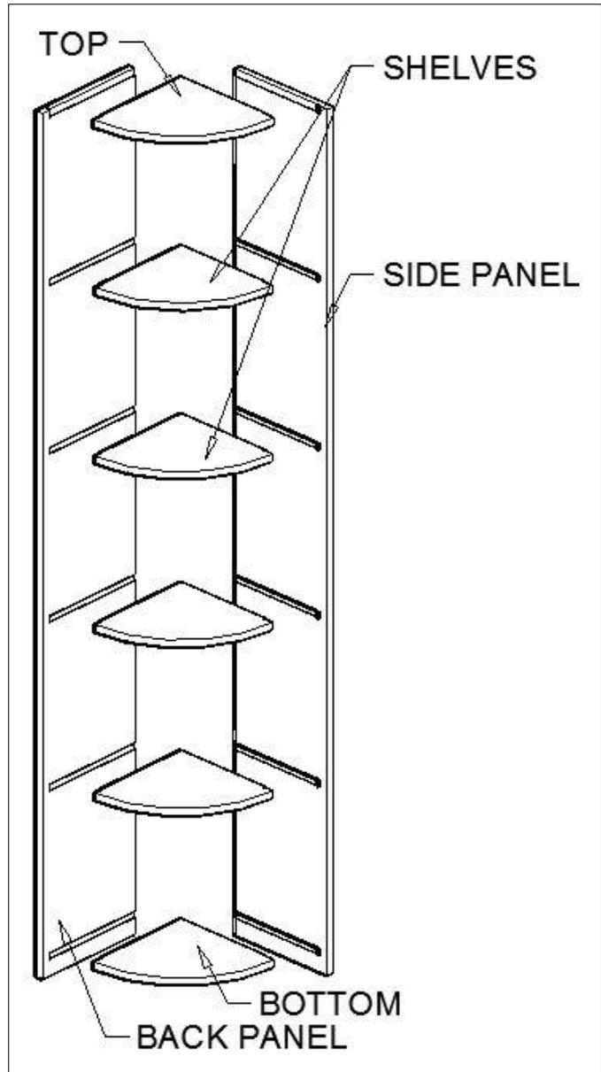
Quarter Round Displays consist of side and back panels, top panel, bottom panel, and shelves. The side panel is applied to the wider back panel. The shelves have a smaller radius than the top and bottom panels which create a 1/4" reveal to the side and back panels.
