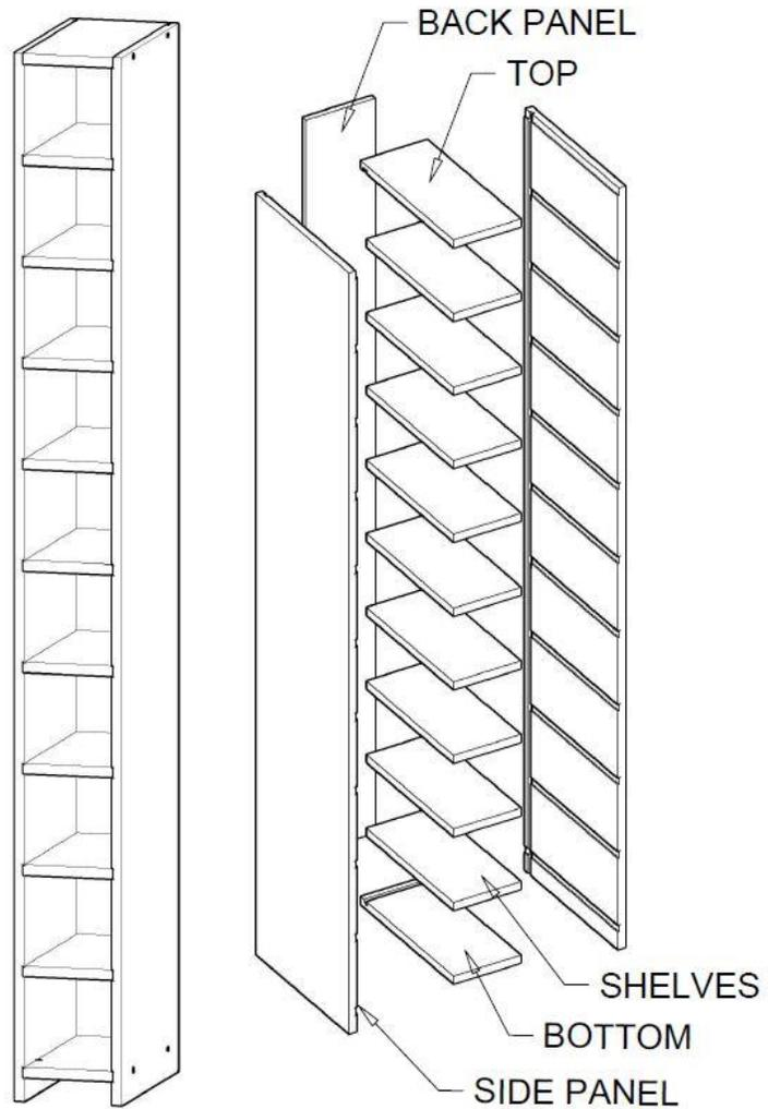
Bottle Cubbies can vary in design based on the aesthetic that was chosen. Some have a solid back panel where others incorporate smaller nailer pieces that attach to the wall. Please familiarize yourself with the parts in the images above for the cubbie you are assembling. The following instructions will detail the assembly of a Bottle Cubbie with nailers and will make references to the solid backed panel version as needed.
