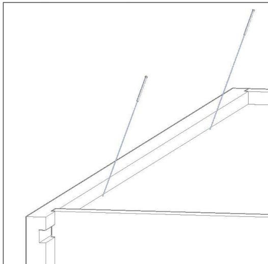
7. Turn the unit onto its back and apply the side face frame pieces by bradding them to the front of the unit (See Figure 41). **Note: Trimming the top and bottom pieces is typically required.**
