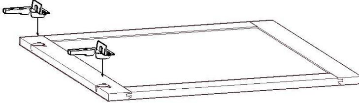
Figure 61: Snap Wing Plates toward Door Interior
