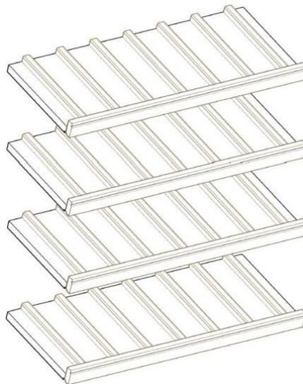
Vertical and Angled Vertical Displays are similar except as the name suggests, an Angled Vertical Display has slotted shelves that get angled at the time of installation. Both have adjustable shelves, a captured back panel, and face frame.
