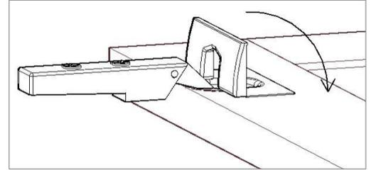
9. Hang the door on the cabinet by pivoting the hinge arms over the wing plates (See Figure 62).
