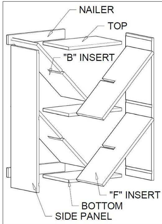
These two components are very similar in construction and have been grouped together to minimize redundancy. Please familiarize yourself with the parts in the images above. The instructions will detail the assembly of a Solid Rectangular Bin and call out the Diamond Cube steps as needed.
