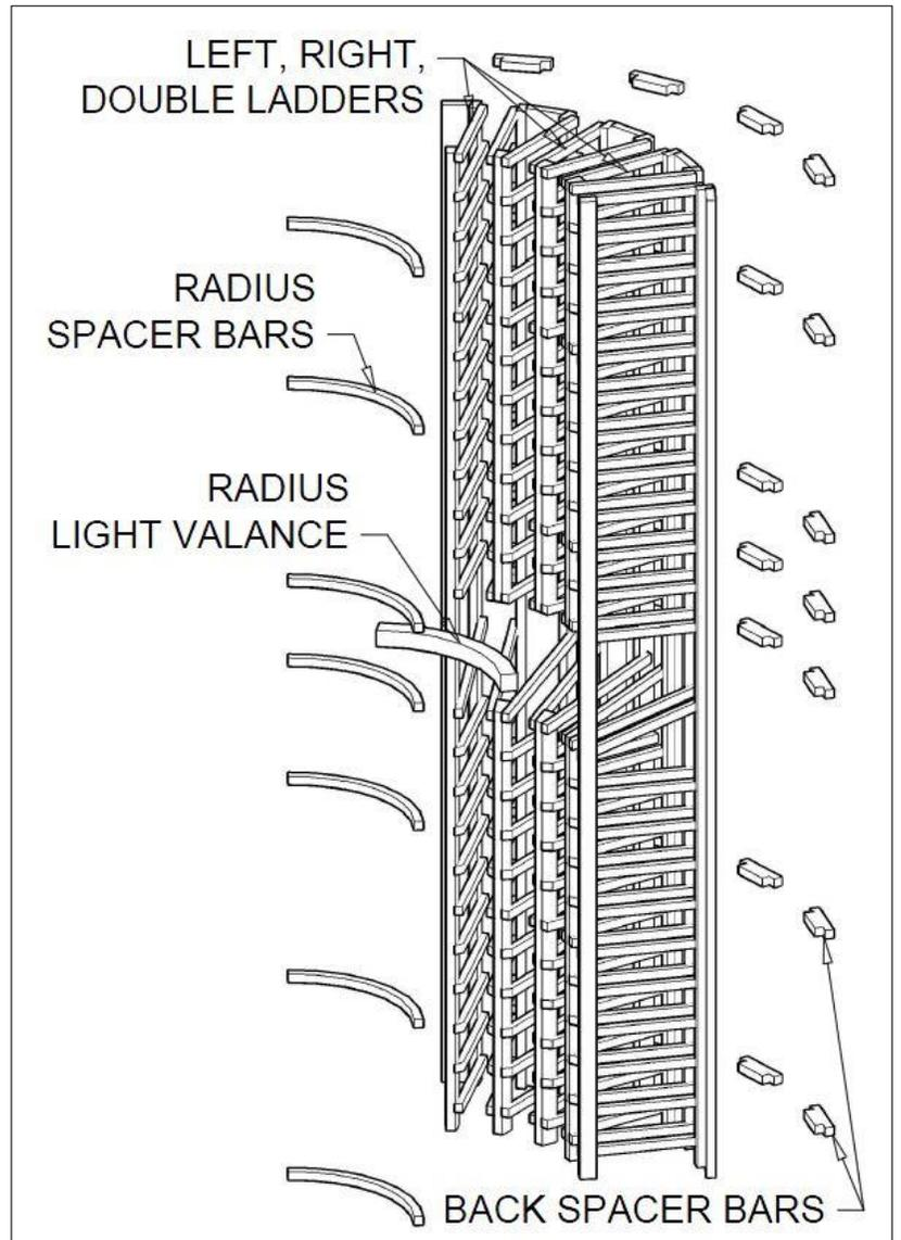
Vigilant Radius Racks are a bit challenging and not recommended for beginners. We suggest that you familiarize yourself with Vigilant’s straight ladder racking before tackling this item. The radius rack includes left, right and double ladders, radius and back spacer bars and a radius light valance. It’s important to note that this item will require cutting the radius spacer bars to the proper size for assembly.
