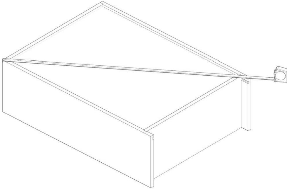
6. Fix the back panel into place by bradding at an angle through the back panel into the side panels. This should be done as needed on each vertical and horizontal edge (See Figure 40). Be careful not to brad through the side panel. Also, verify the cabinet's overall width before bradding the opposing side to make sure it will fit.
