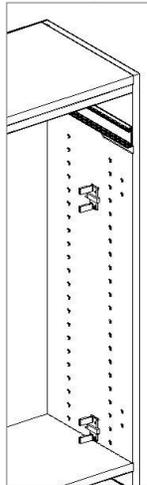
Figure 59: Snap Wing Plates Toward Side Panel
