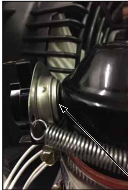
**NOTE:** Make sure the surface of the thermal switch is located at the ridge of the receiver, and is making good contact.
