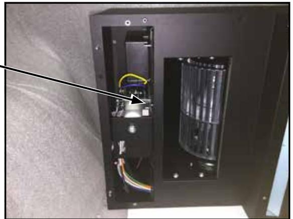
**25** Re-install the electrical panel using the 2 Phillips head screws removed in step #6.
