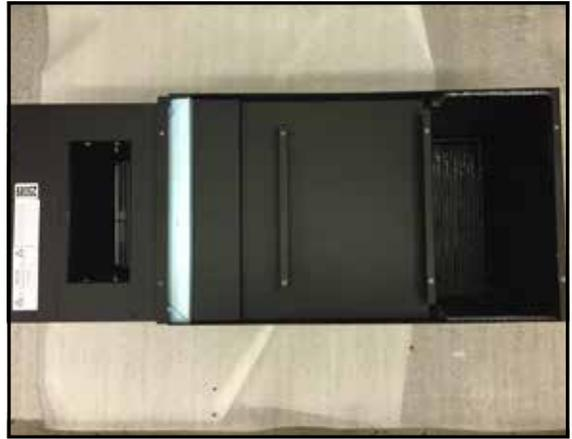
**6** Locate the electrical panel access door, and remove the two Phillips head screws. (Set screws and panel aside for later use)
