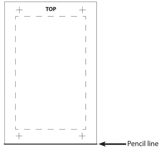
3. Use a 5/16" drill bit to drill a hole in the center of each cross (+).
