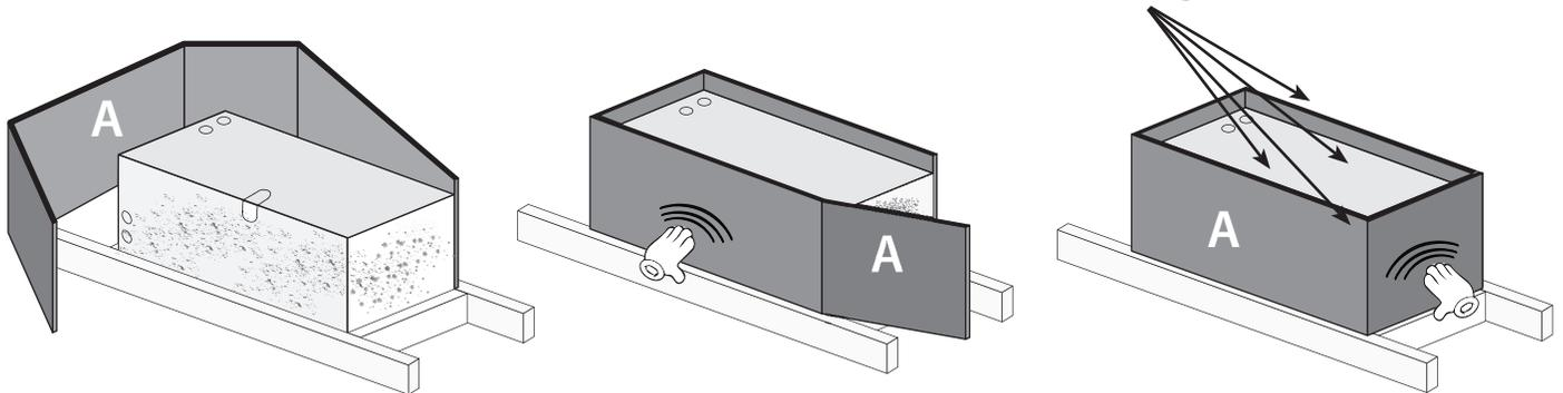
4. Set insulation in place by pressing firmly on all surfaces of the insulation that come in contact with the sides of the evaporator unit (see illustration).
