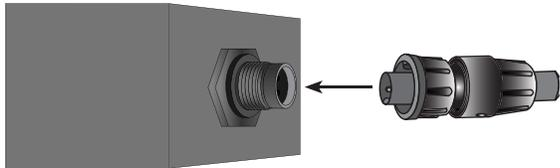
20. Connect the end of the display cable labeled "UNIT" to the wire labeled "UNIT" coming from the electrical box.
