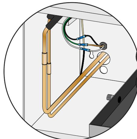
13. Connect power supply wires to the pre-installed butt splice connectors located inside of the unit (hot=black, neutral=white, ground=green).
