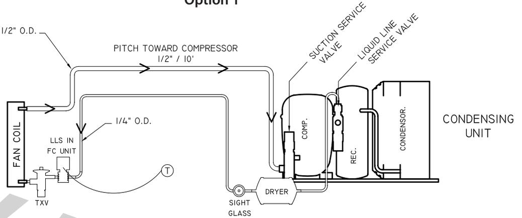
**SINGLE FAN COIL PIPING SYSTEM**
