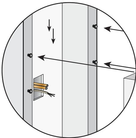
11. Remove the line set caps. Route the 3/8" suction line and 1/4" liquid line into the unit and braise.
