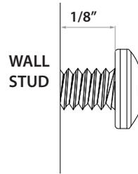
7. Install the supplied four (4) 2" #8 hex-head screws at the locations marked, leaving 1/8" between the wall surface and screw head.
