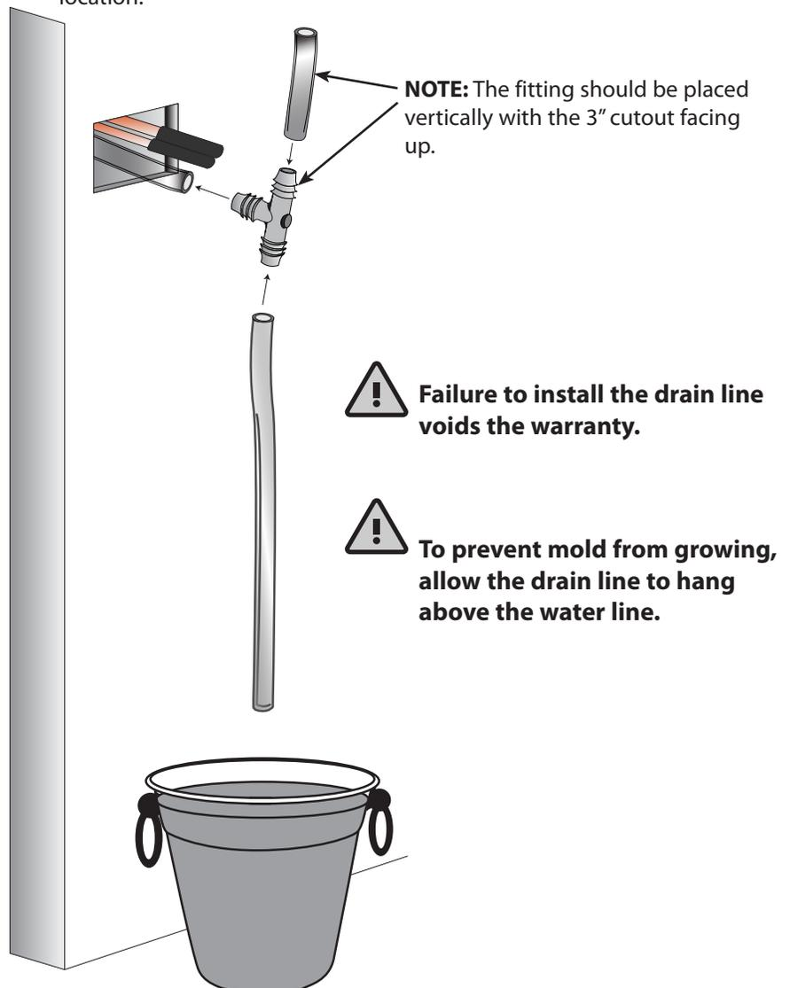
**NOTE:** The fitting should be placed vertically with the 3" cutout facing up.
