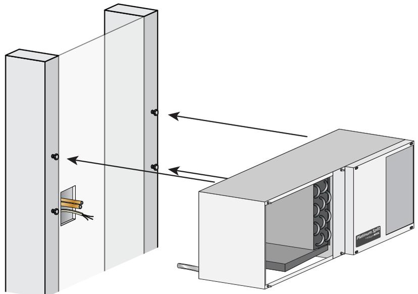
10. Using a ¼" wrench or socket, tighten the accessible mounting screws on the left-hand side of the interior of the unit.
