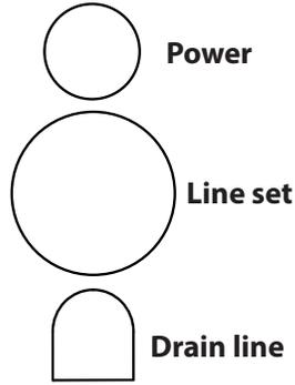
1. Remove the knockouts for the drain line, line set, and electrical on the bottom or rear of the unit (depending on your installation location).
