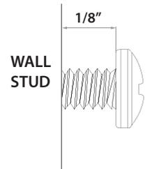
5. Install the four (4) supplied 1¾" hex head screws into the studs at the locations marked leaving ⅛" between the wall surface and screw head.
