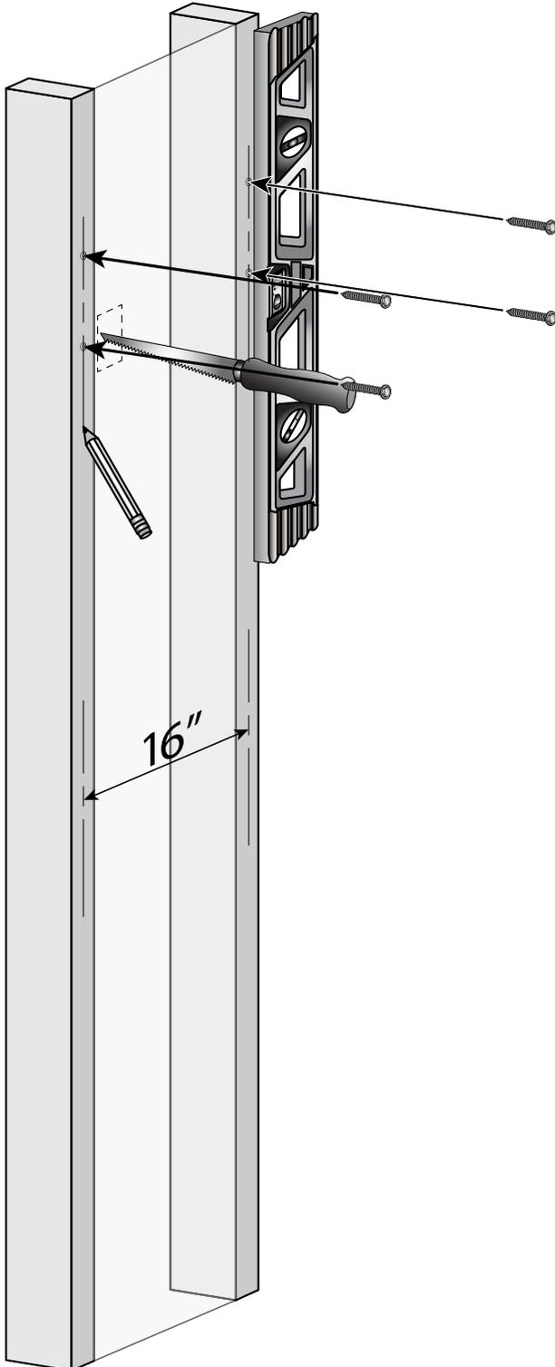
**Note:** The top of the unit must be installed a minimum of 6" and a maximum of 18" from the ceiling.
