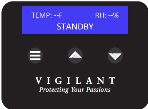
The Guardian sensor requires an initial stabilization period when first powered. At this time, the control will run a stabilization program.
